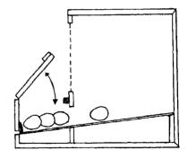
Figure 23: Cross-section of roll-away nest
