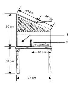
Figure 20: Communal laying nest 1. entrance 2. retaining board
