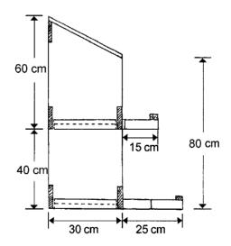
Figure 22: Cross-section of individual laying nests
