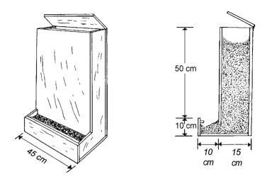
Figure 14: Rectangular wooden feeder
