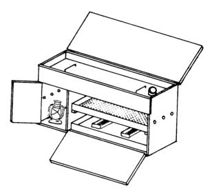
Figure 6: Kerosene incubator with internal heat source.
