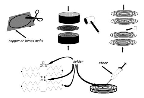
Figure 10: How to make a double ether capsule.
