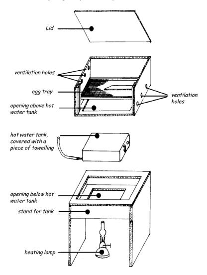
Figure 2: Incubator with kerosene lamp heating.
