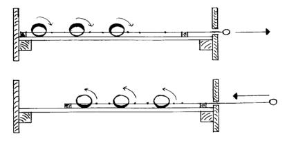
Figure 3: Egg-turning device.
