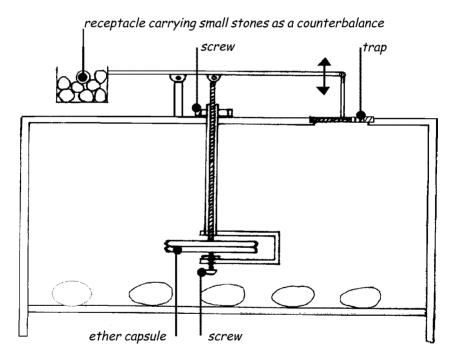
Cold: the trap closes, warm air is trapped inside the incubator Hot: the trap opens, warm air escapes.
