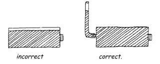
Figure 5: Filling the tank.
