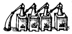
The first type of still was called an Alembic, although this properly referred to the cap with a spout that sat on top of the boiling vessel. It worked well, and with variations to make use of modern materials is just what you need to distill botanicals. The second is reminiscent of the moonshine contraptions still used (and raided) in America, but without the cooling 'worm' so characteristic of them.
