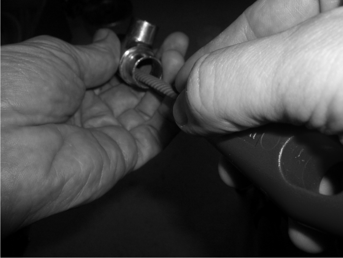
Photo #3. Removing the end stop shoulder.
