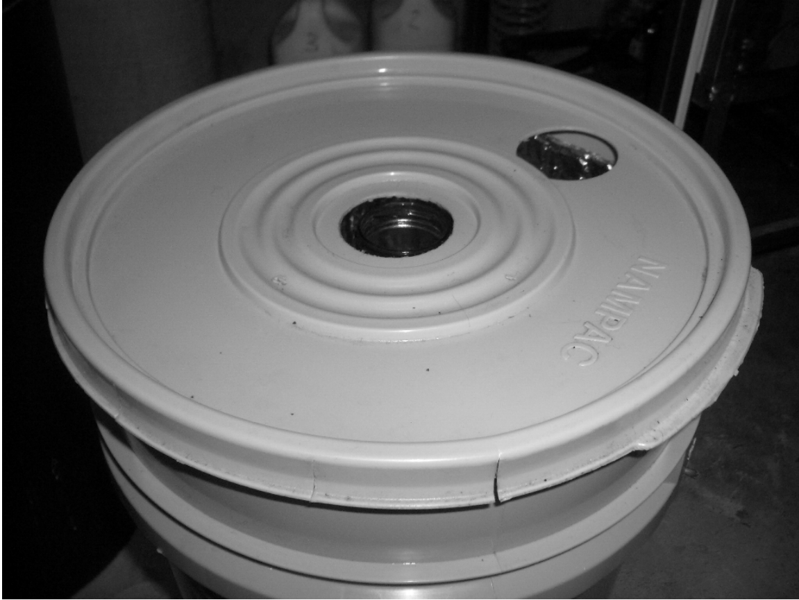
Photo #1. Top of Liquid trap containment vessel.
