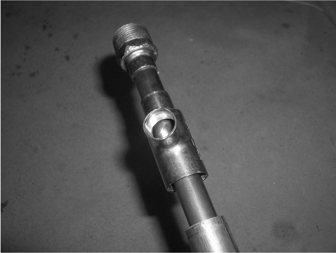
Photo #4. Top end of coaxial drier showing water jacket connection in exploded view.
