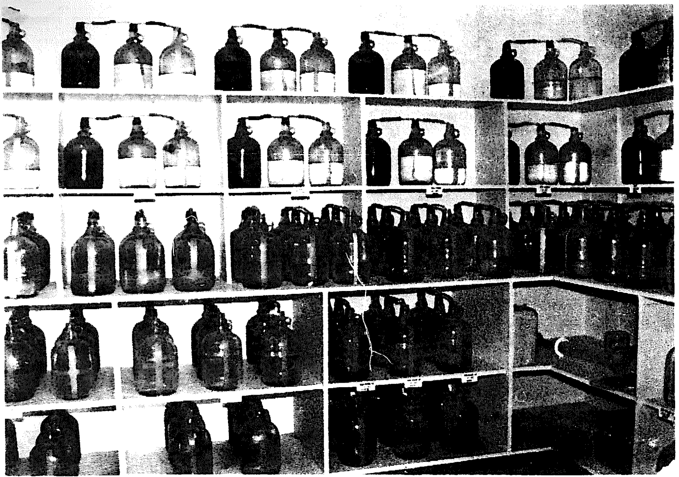
Illustration 1-4: Experimental laboratory digesters at Maya Farms
